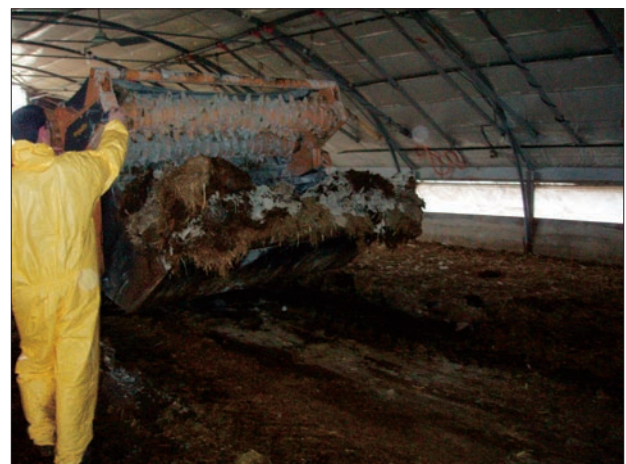
Figure 1: Example of homogenisation of litter and lime inside using standard mixing equipment (Ain – France)
